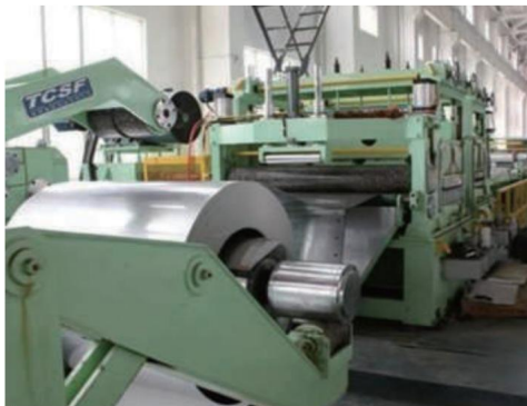
H1:台湾“腾麒”热轧2050中板横剪机 "TCSF" HR 2050MM Cut- To-Length LINE
