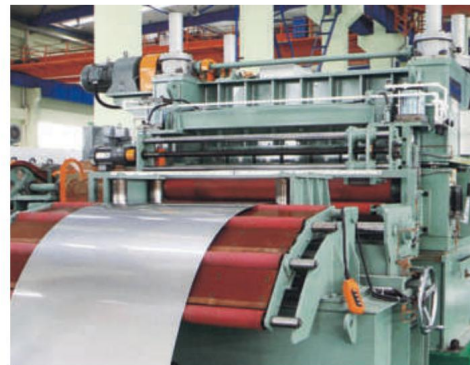
L1:韩国“大铤”冷轧1550横剪机 "DAEHYUN" CR 1550mm CTL Line
